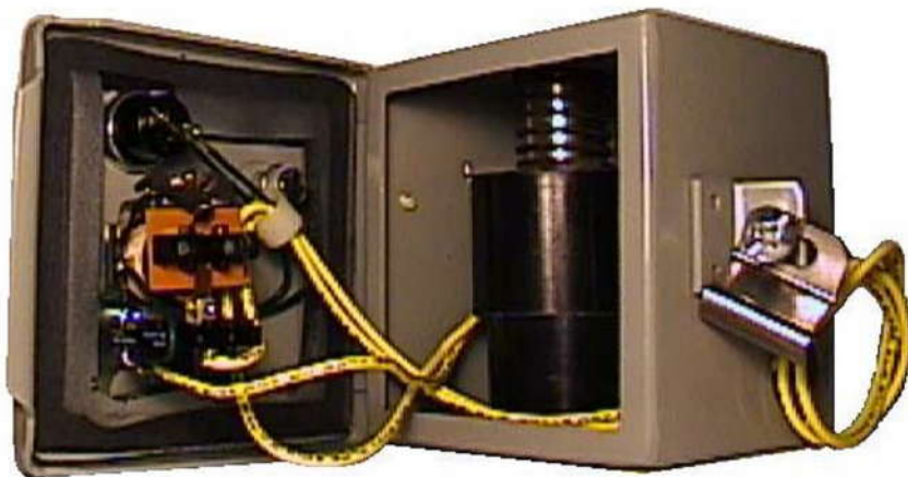
Photo of Internal Coil Housing Detail
