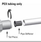
3. If using PEX tubing, insert pipe stiffener (provided) into end of pipe.
