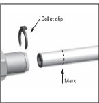
4. Push tubing into tailpiece up to mark.5. Insert collet clip.
