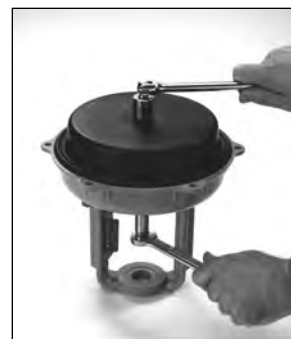
Fig 6 - Replace Washers, Tighten Stem Nut
