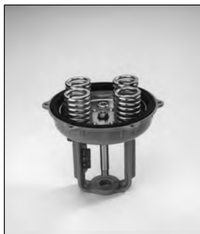
Fig 2A - Remove Upper Housing to Expose Springs (4 Shown)
