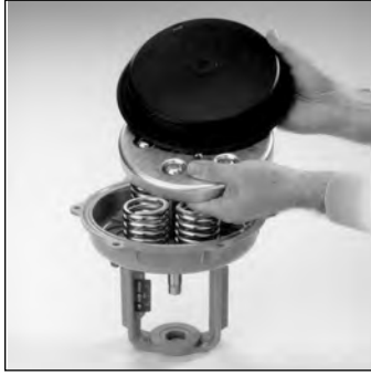
Fig 2C - Remove Diaphragm, Thrust Plate
