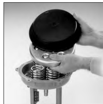
Fig 3 - Remove Diaphragm (Leave Thrust Plate On).
