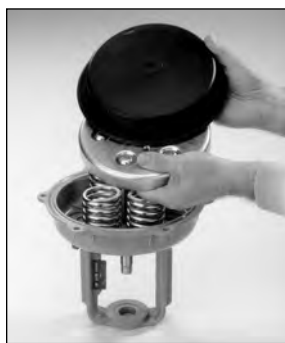
Fig 2B - Remove Diaphragm and Thrust Plate
