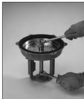
Fig 2B - Remove Springs, Stem Nut
