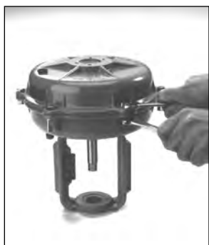
Fig 1 - Remove Housing Bolts
