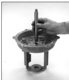
Fig 4 - Remove and Replace Stem
