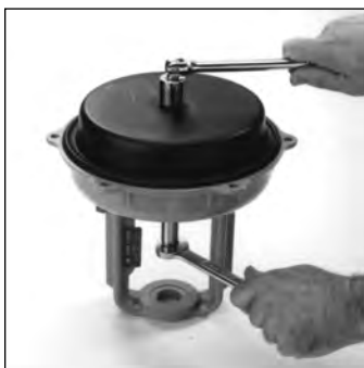
Fig 2 - Remove Stem Nut, and Washers
