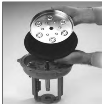
Fig 4 - Remove Thrust Plate and Old Diaphragm
