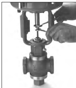
Fig 3 - Loosen Stem Locknuts
