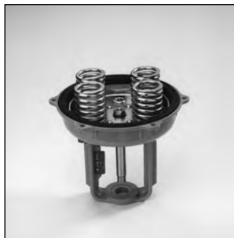
Fig 2 - Remove Upper Housing, Remove Springs (4 Shown)
