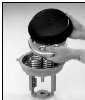
Fig 5 - Replace Springs, Reversed Thrust Plate and Diaphragm
