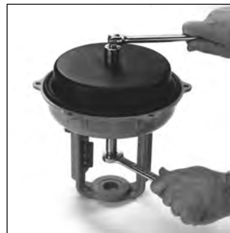
Fig 2B - Remove Stem Nut, & Washers
