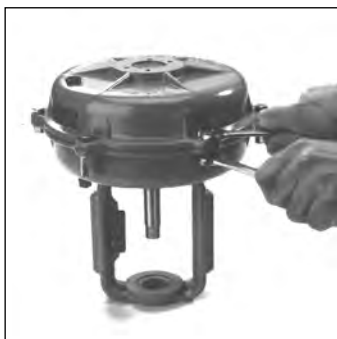
Fig 1 - Remove Housing Bolts
