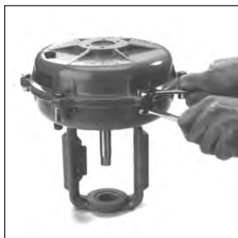
Fig 1 - Remove Housing Bolts
