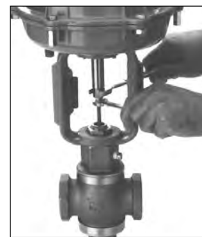
Fig 3 - Loosen Stem Locknuts
