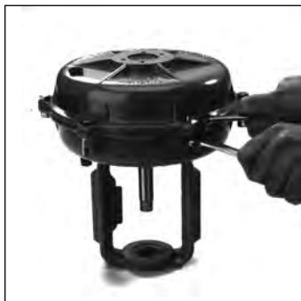
Fig 1 - Remove Housing Bolts (extended versions last and gradually)
