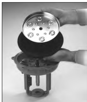
Fig 5 - Reverse Replacement of Diaphragm and Thrust Plate
