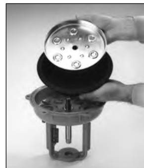
Fig 2C - Remove Washers, Thrust Plate, Diaphragm
