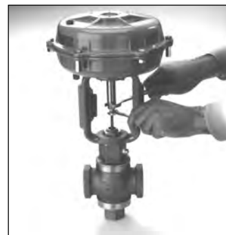
Fig 1 - Rotate Lock Nuts to Adjust Preload
