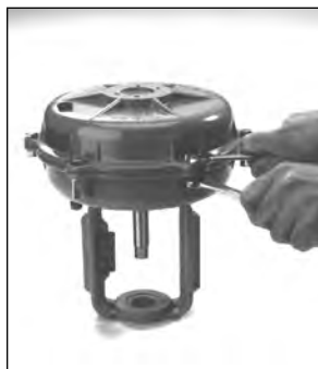
Fig 1 - Remove Housing Bolts
